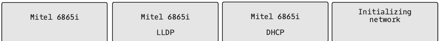
During the first start up, the 6865i phone attempts to contact the Redirection and Configuration Server for current server information. No personal information is transmitted from the phone during this process.
