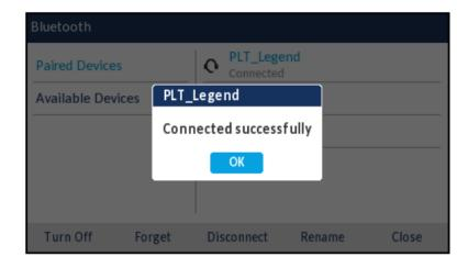
To disconnect a device, press the Disconnect S-key and proceed by clicking Yes.
