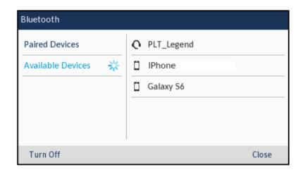
Press the right navigation key to move to the Bluetooth device selection column.
