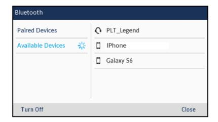
Press the right navigation key to move to the Bluetooth device selection column.
